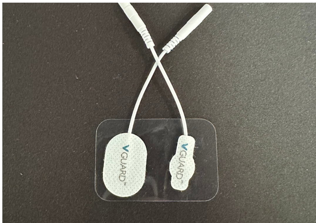
Fig. 5. VGuard Electrodes (from left to right) - 1. Larger electrode (outside the ear canal); 2. Smaller electrode (inside the ear)
