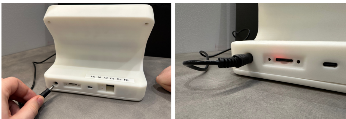
Fig. 9. Connecting the Power to the Base Station
