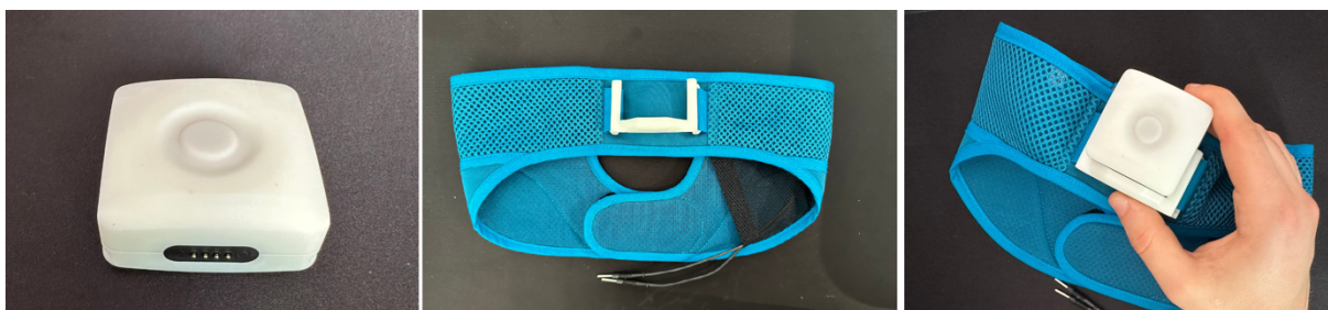
Fig. 3. Illustration of the method of mounting the stimulator in the headband frame and the headband with the stimulator correctly mounted and without the stimulator
