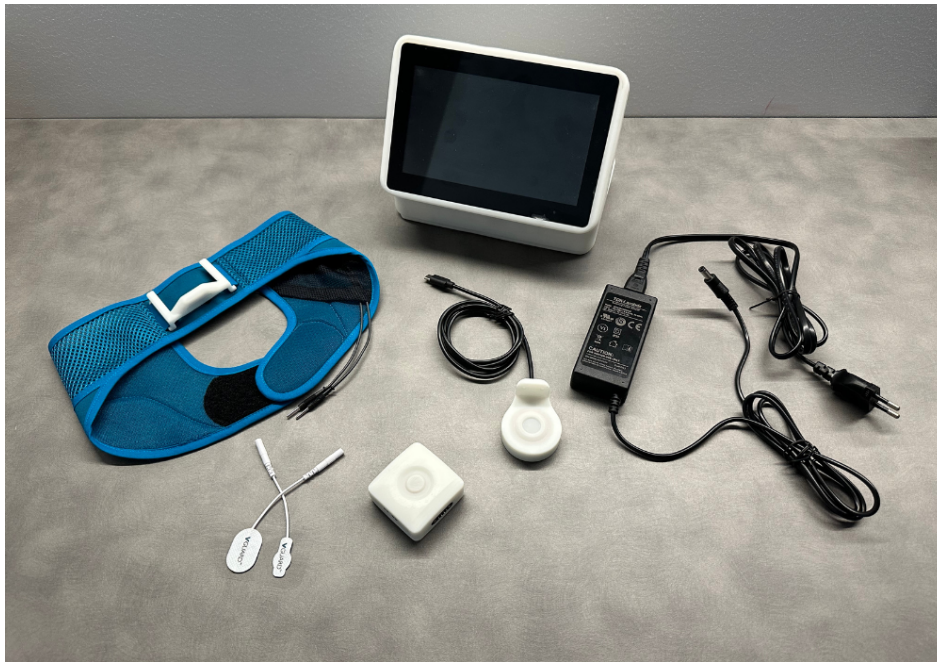
Fig. 1. VGuard System (from left to right) - 1. Headband, 2. Electrodes, 3. Stimulator, 4. Base Station, 5. Charger, 6. Power Supply
